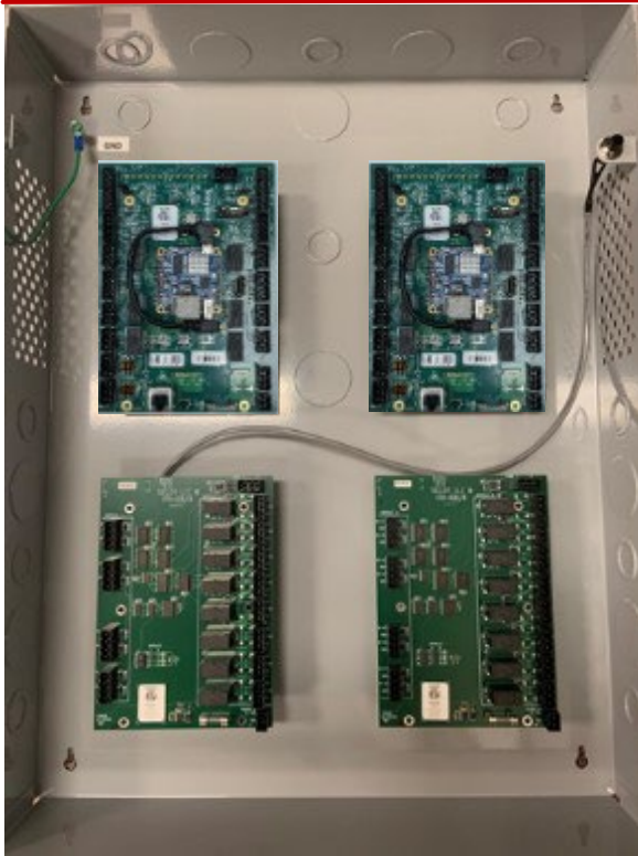
The 2700 includes 4 supervised or unsupervised inputs and 4 auxiliary outputs with field replaceable relays, expandable via daisy chain up to four 170 I/O expansion boards per 2700 controller.
