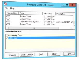
**Door List Control** – Allows operators to take actions on doors without having to launch Pinnacle on the Desktop. Operators can manage a list of doors for selected actions such as lock, unlock, or momentary unlock. Originally built for 911 call center that needs to have multiple windows open at once. Even when minimized on toolbar, events will continue to be displayed.
