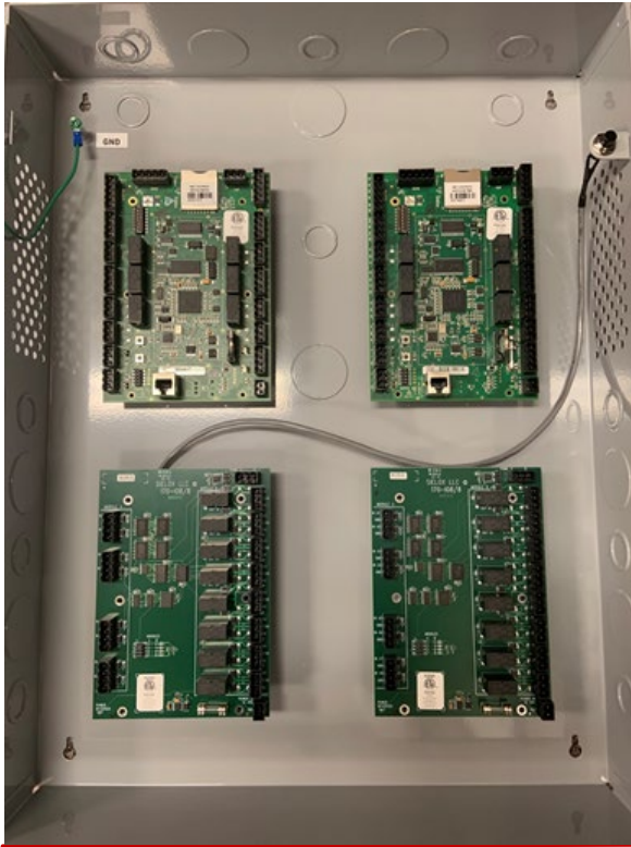
The 1700 includes 4 supervised or unsupervised inputs and 4 auxiliary outputs with field replaceable relays, expandable via daisy chain up to two 170 I/O expansion boards per 1700 controller.
