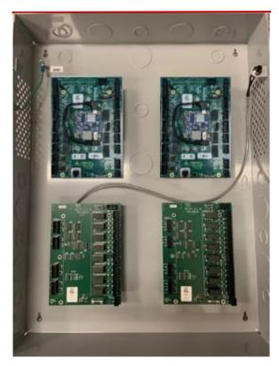
The 2700 includes 4 supervised or unsupervised inputs and 4 auxiliary outputs with field replaceable relays, expandable via daisy chain up to two 170 I/O expansion boards per 2700 controller.
