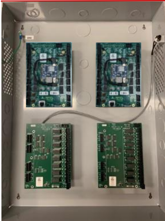
The 2700 includes 4 supervised or unsupervised inputs and 4 auxiliary outputs with field replaceable relays, expandable via daisy chain up to two 170 I/O expansion boards per 2700 controller.
